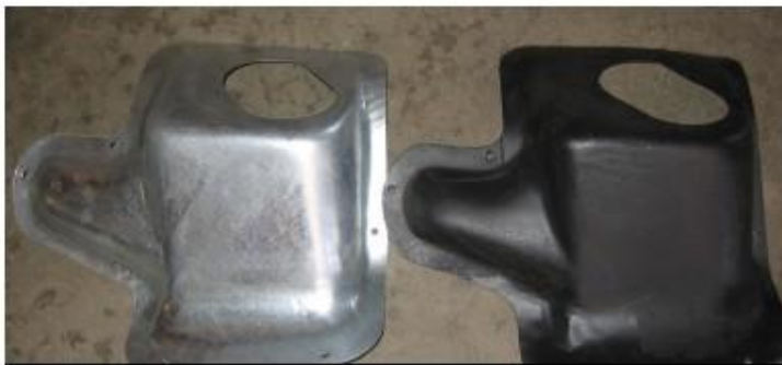
A side by side comparison of the Dearborn Classics reproduction tunnel hump (left) and an original 1963 4-speed tunnel hump removed from a 1963 V-8 Ranchero.
