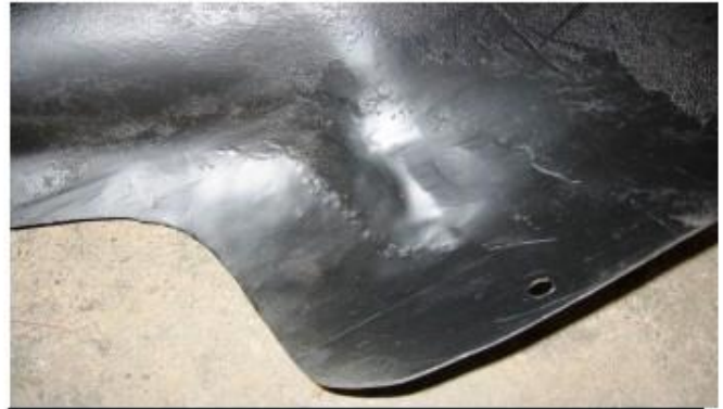
A repair made to an original tunnel hump. The multiple contours make it difficult to patch.
