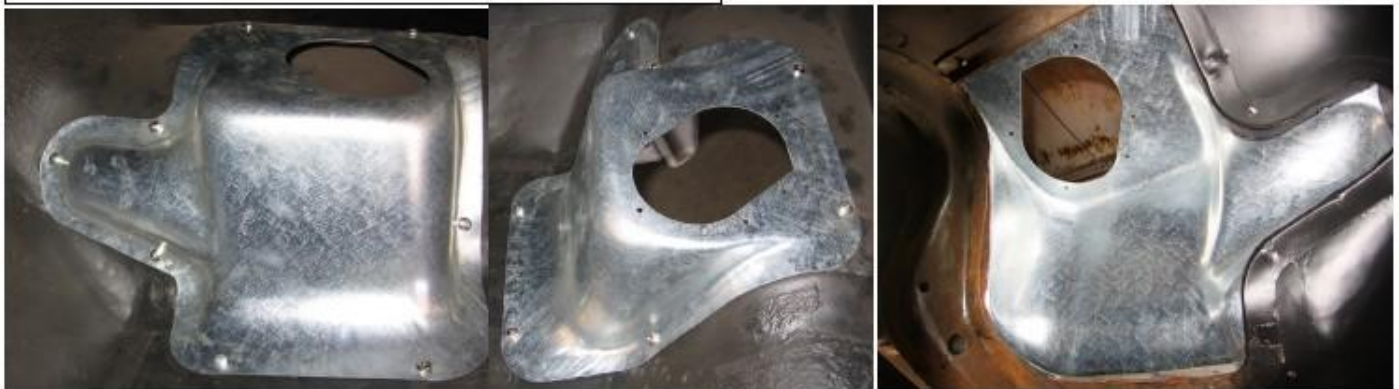
Three different views of the new Dearborn Classic Tunnel Hump Installed; the view on the left is looking in from the drivers door, the center view is looking down from above and the view on the right is looking up from below.
